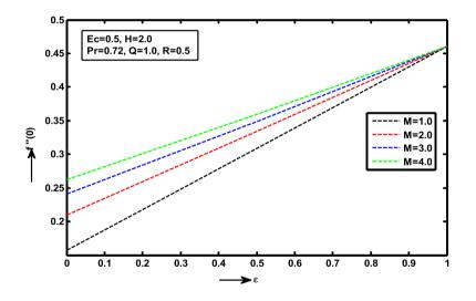
Fig. 10. Skin friction coefficient for various values of M.
