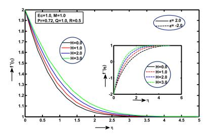
Fig. 3a. Velocity profiles for various values of H.
