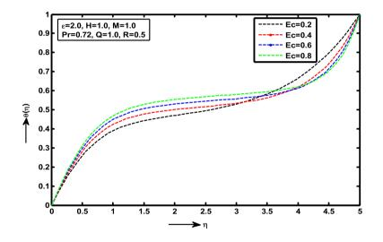
Fig. 5. Temperature profiles for various values of Ec.
