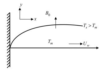
Fig. 1. Boundary layer on moving continuous surface.
