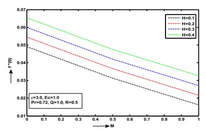
Fig. 9. Skin friction coefficient for various values of H.
