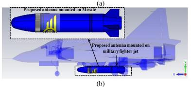
**Figure 6**. The geometry of (a) conformal WSP antenna, (b) WSP antenna mounted on aircraft with a guided missile.
