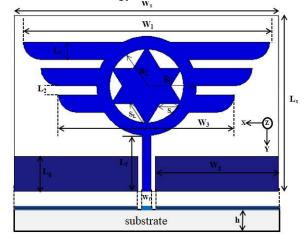
Figure 1. The geometry of the wing-shaped patch (WSP) antenna.
