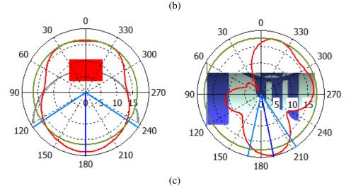
Figure 9. E-field and H-field radiation patterns of conformal WSP antenna (a) 7 GHz, (b) 10.24GHz, (c) 16.16GHz frequencies.
