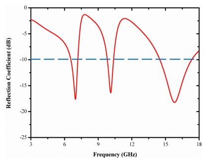
Figure 2. S<sub>11</sub>of wing-shaped patch (WSP) antenna.
