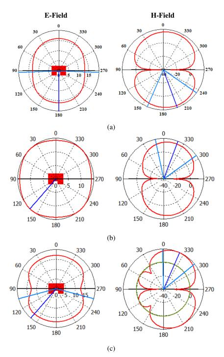
**Figure 5**. E-field and H-field radiation patterns of WSP antenna at (a) 6.97 GHz, (b) 10.12GHz, (c) 15.78GHz frequencies
