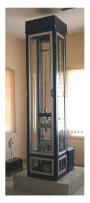
Figure 1 Instrumented falling-weight impact test equipment.
