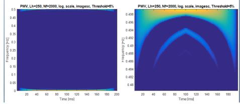
Figure 5. pseudo-WVD spectrum of the received signal (image to the right is the magnified version of spectrum's positive peak)
