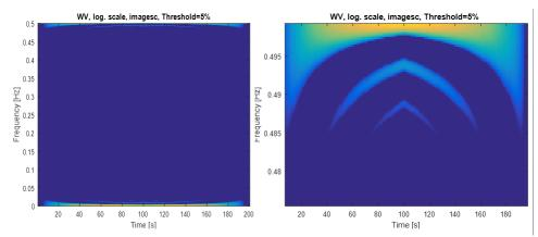
Figure 4. WVD spectrum of received signal (image to the right is the magnified version of spectrum's positive peak)
