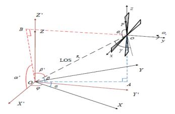
Figure 1. Rotor in Radar coordinate system
