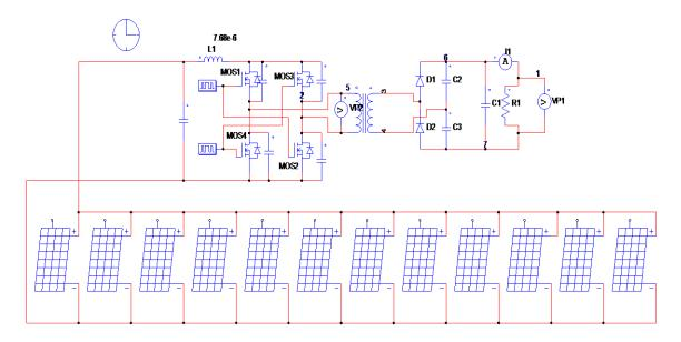
Figure 1. A Current Fed DC-DC Converter topology with voltage doubler rectifier in the output
