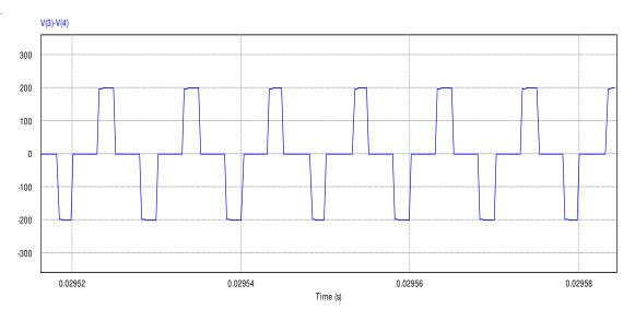
Figure 6. Output voltage at transformers secondary terminal
