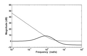
**Fig. 15.** Magnitude plot of complementary sensitivity function  $T_d(j\omega)$  (solid),  $1/l_m(j\omega)$  for  $\Delta \tau = -0.5$  (dot).
