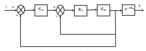
Fig. 2. Block diagram representation of servo response.
