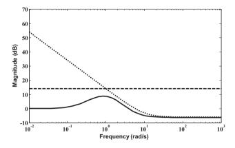
**Fig. 14.** Magnitude plot of complementary sensitivity function  $T_d(j\omega)$  (solid),  $1/l_m(j\omega)$  for  $\Delta \theta_p = 0.25$  (dot),  $1/l_m(j\omega)$  for  $\Delta k = 0.2$  (dash).
