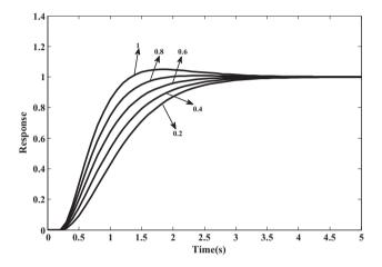
Fig. 8. Servo response of Example 1 for various set point weighting parameters.
