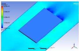
Figure 11. Velocity contour of model with pencil column along z-axis
