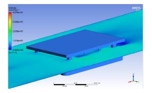
Figure 8. Velocity contour of model with pencil column (-) x axis
