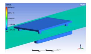
Figure 12. Pressure contour of model without pencil column
