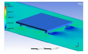
**Figure 7.** Velocity contour of model without pencil column (+) x axis.
