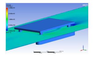
**Figure 6.** Velocity contour of model without pencil column along (-) x axis
