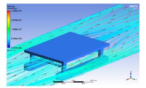
Figure 14. Streamline contour of model without pencil column
