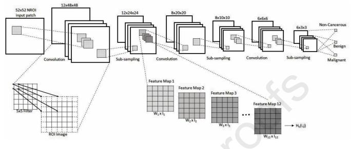
Figure 4: Structure of the DCNN
