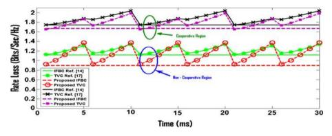
**Fig. 4** Rate loss versus sub-frame index  $T_s$  when  $B_{res} = B_{res,TVC} = 8$ ,  $\tau_{l,i,i} = 5$ ,  $\tau_{l,i,j} = 10$ ,  $\eta_{l,i,i} = -\eta_{l,i,j} = 0.99$  and  $\gamma_{l,i,i}$ ,  $\gamma_{l,i,j}(r_i, r_j = 500) = 10$  dB
