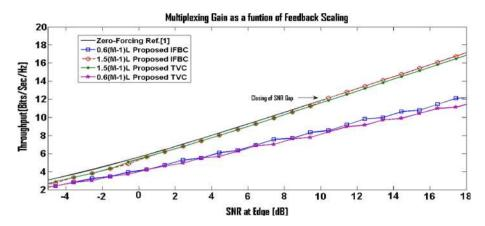
**Fig. 8** Feedback scaling for multiplexing gain when  $\tau_{l,i,i} = \tau_{l,i,j} = 2$ ,  $\eta_{l,i,i} = \eta_{l,i,j} = 0.99$
