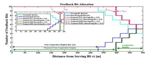
**Fig. 2** Feedback allocation strategy for IFBC for various  $\varepsilon$  when  $\gamma_{l,i,i}$  ( $r_i = 500$ ) = 10 dB and  $\gamma_{l,i,i}$  ( $r_i = 500$ ) = 10 dB,  $\tau_{l,i,i} = \tau_{l,i,j} = 10$
