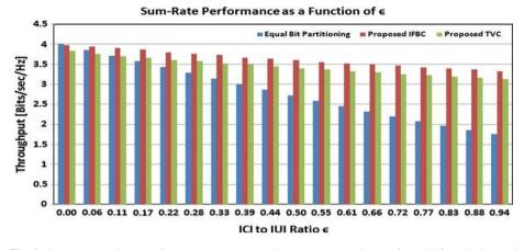
**Fig. 3** Sum-rate against  $\varepsilon$  for  $B_{res} = B_{res,TVC} = 8$ ,  $\tau_{l,i,i} = \tau_{l,i,j} = 2$ ,  $\gamma_{l,i,i} (r_i = 500) = 10 \text{ dB}$  and  $\gamma_{l,i,i} (r_j = 500) = 10 \text{ dB}$
