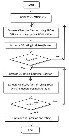
**Figure 2.** Flowchart for optimal rating and position of DG using BFOA
