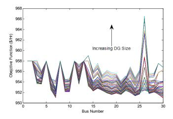
**Figure 4.** Variation of objective function with DG location for IEEE 30 bus system.
