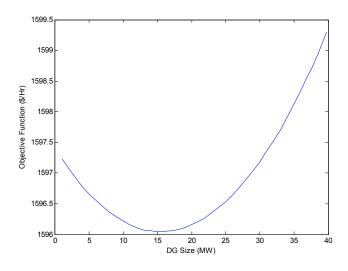
**Figure 5.** Variation of objective function with DG size for IEEE 14 bus system at optimal location (bus no. 13).
