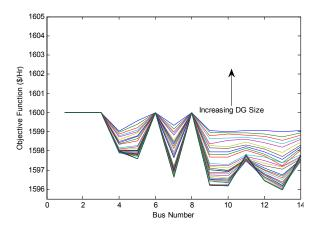
**Figure 3.** Variation of objective function with DG location for IEEE 14 bus system.
