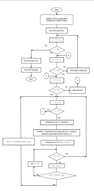
**Figure 1.** Flowchart for Optimal Power Flow using Bacterial Foraging Optimization Algorithm (BFOA-OPF).
