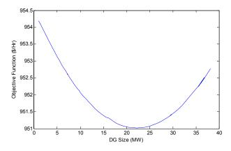
**Figure 6.** Variation of objective function with DG size for IEEE 30 bus system at optimal location (bus no. 7).
