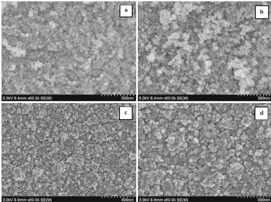
**Figure 11.** Microstructure of Al-doped ZnO thin films for grey theory predicted design at different annealing temperatures, (a) 350, (b) 400, (c) 450 and (d) 500°C.
