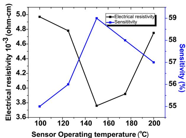
Figure 9. Resistivity and sensitivity plotted as a function of sensor operating temperature for Al-doped ZnO thin films at the annealing temperature of 450°C.
