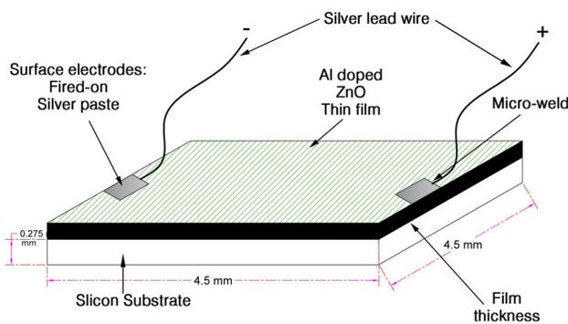
**Figure 3.** Schematic of CO gas sensing.
