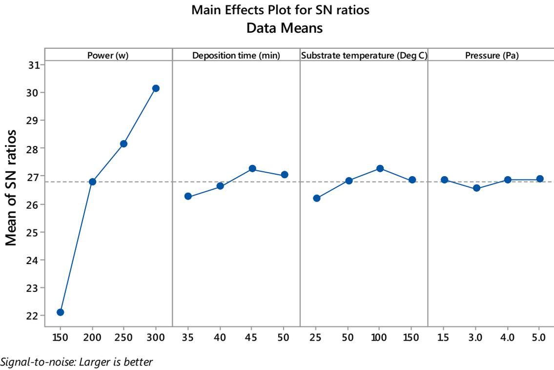
Figure 5. S/N ratio response curve for deposition rate.
