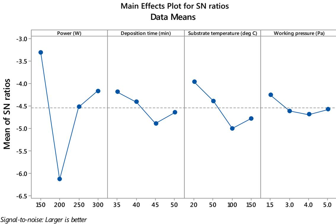
**Figure 7.** S/N ratio response curve for grey relation grade.
