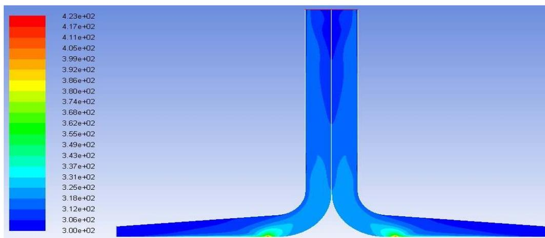
**Figure 3a.** Temperature contour maps of SUT plant at 600  $\text{Wm}^{-2}$  at 5° canopy value angle.
