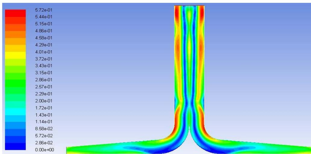
**Figure 4b.** Velocity contour maps of SUT plant at  $800 \text{ Wm}^{-2}$  at  $5^\circ$  canopy angle
