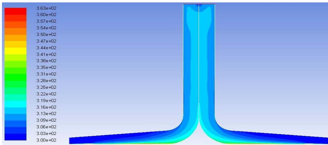
**Figure 3c.** Temperature contour maps of SUT plant at  $1000 \text{ Wm}^{-2}$  at  $5^\circ$  canopy angle.
