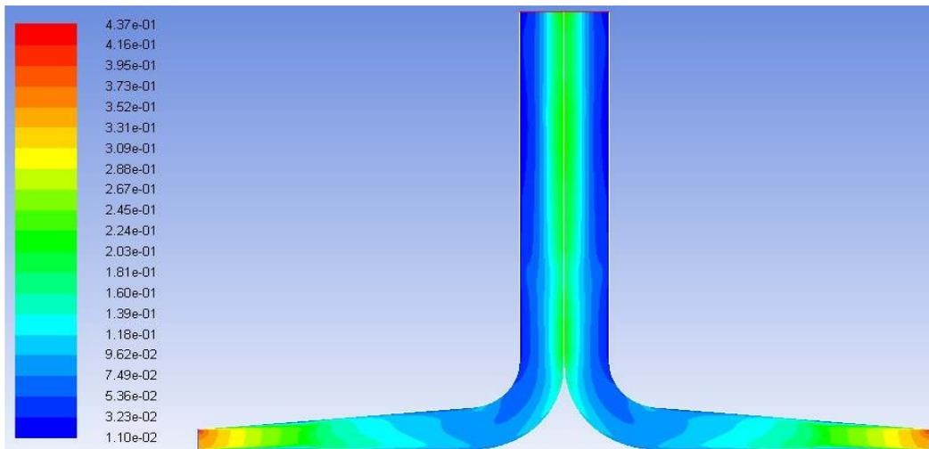
**Figure 2b.** Pressure contour maps of SUT plant at  $800 \text{ Wm}^{-2}$  at  $5^\circ$  canopy value.
