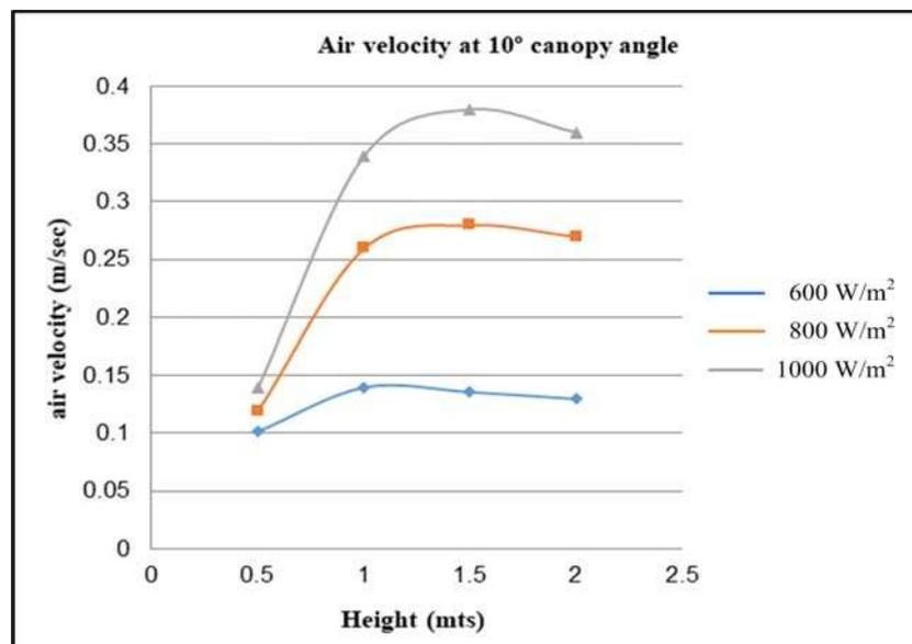
**Figure 8b.** Air velocity vs Height at 10° canopy angle.
