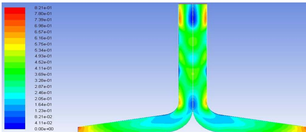
**Figure 7b.** Velocity contour maps of SUT plant at  $800 \text{ Wm}^{-2}$  at  $10^\circ$  canopy angle.
