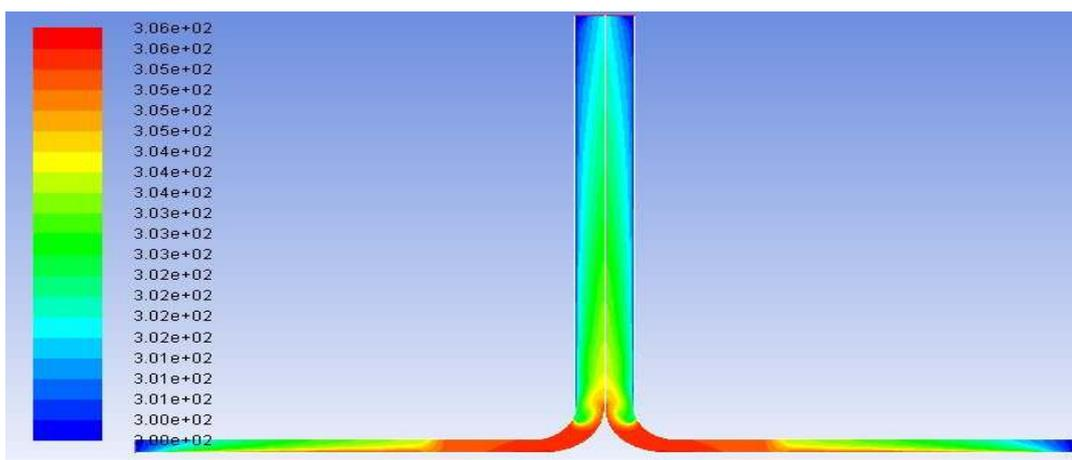
**Figure 1b.** Temperature contour maps of SUT at 0° canopy angle and 600 Wm<sup>-2</sup>.
