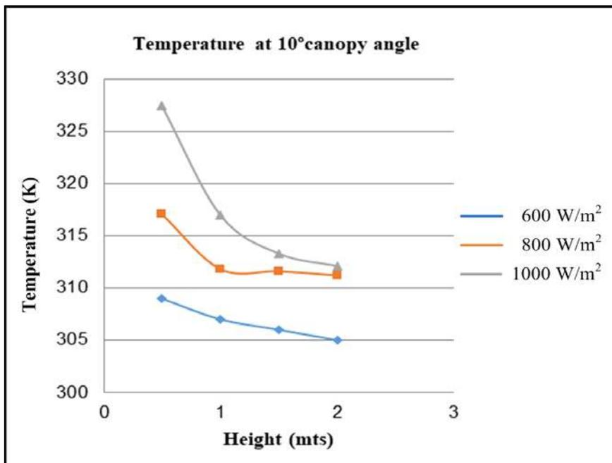
**Figure 9b.** Temperature vs Height at 10° canopy angle.
