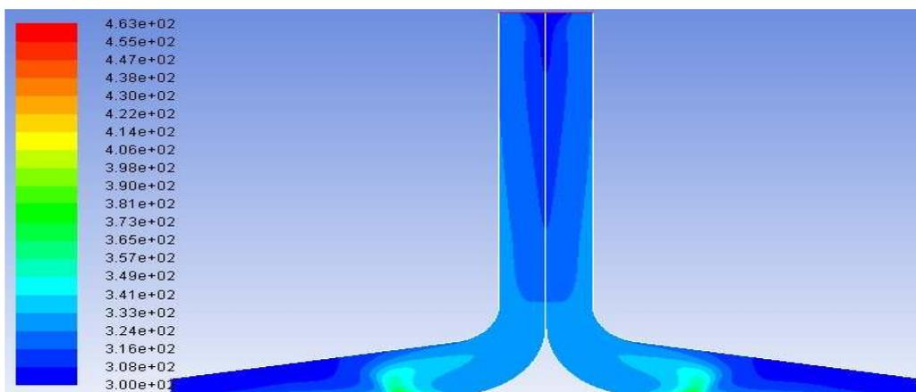
**Figure 6c.** Temperature Contour maps of SUT plant at  $1000 \text{ Wm}^{-2}$  at  $10^\circ$  canopy angle.
