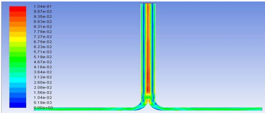
**Figure 1c.** Air velocity contour maps of SUT 0° canopy angle and 600 Wm<sup>-2</sup>.
