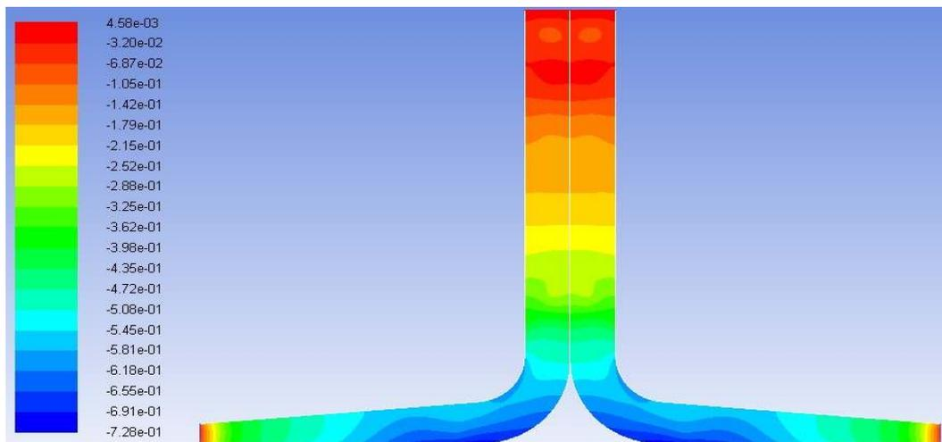
**Figure 2a.** Pressure contour maps of SUT plant at 600 Wm<sup>-2</sup> at 5° canopy value.
