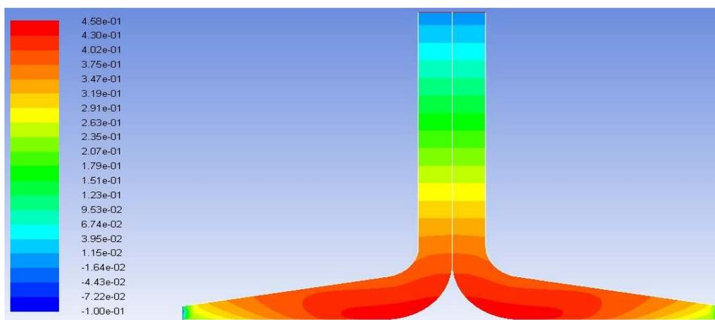
**Figure 5a.** Pressure contour maps of SUT plant at  $600 \text{ Wm}^{-2}$  at  $10^\circ$  canopy angle.
