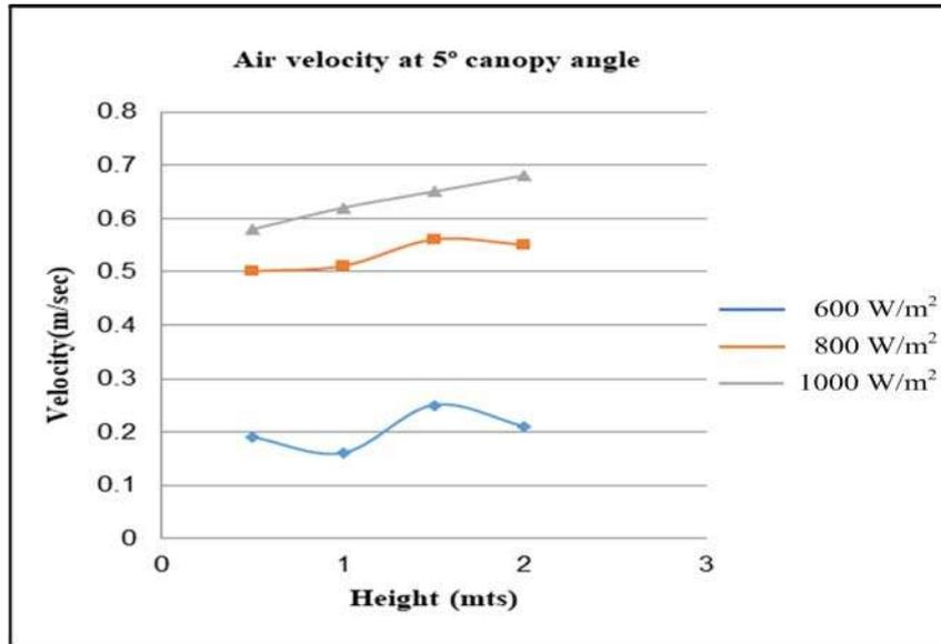
**Figure 8a.** Air velocity vs Height at 5° canopy angle.
