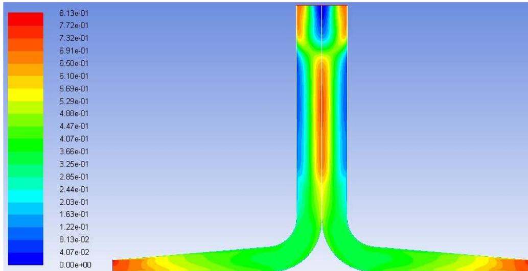
**Figure 4a.** Velocity contour maps of SUT plant at  $600 \text{ Wm}^{-2}$  at  $5^\circ$  canopy angle.
