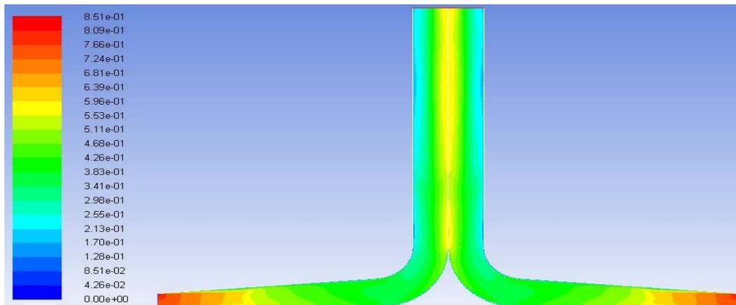
**Figure 4c.** Velocity contour maps of SUT plant at  $1000 \text{ Wm}^{-2}$  at  $5^\circ$  canopy angle.
