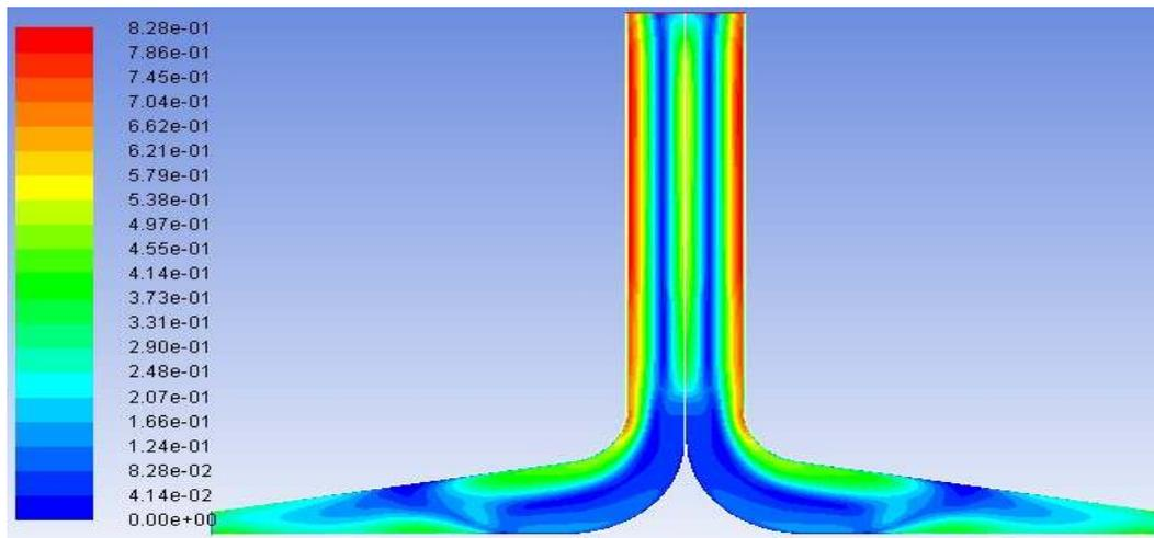
**Figure 7c.** Velocity contour maps of SUT plant at  $1000 \text{ Wm}^{-2}$  at  $10^\circ$  canopy angle.
