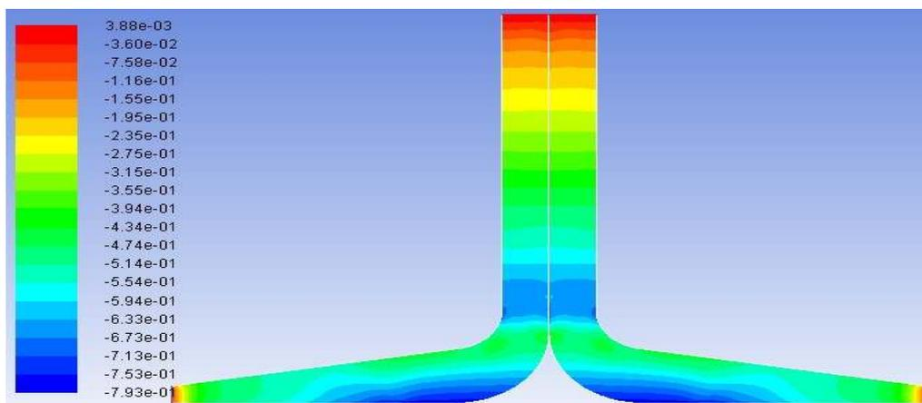
**Figure 5c.** Pressure contour maps of SUT plant at  $1000 \text{ Wm}^{-2}$  at  $10^\circ$  canopy angle.
