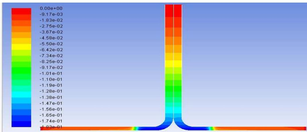
**Figure 1a.** Pressure contour maps of SUT at 0° canopy angle and 600 Wm<sup>-2</sup>.
