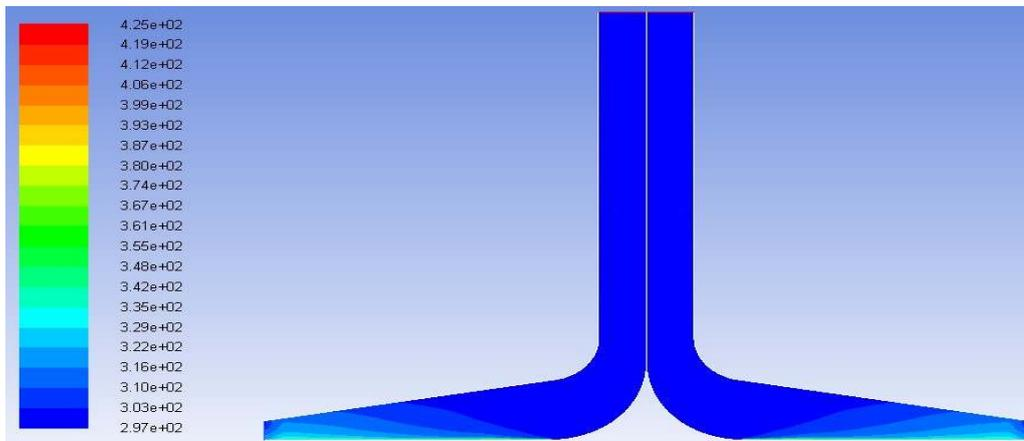
**Figure 6a.** Temperature Contour maps of SUT plant at  $600 \text{ Wm}^{-2}$  at  $10^\circ$  canopy angle.
