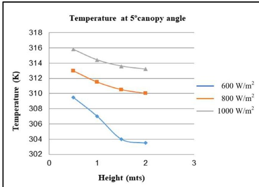
**Figure 9a.** Temperature vs Height at 5° canopy angle.
