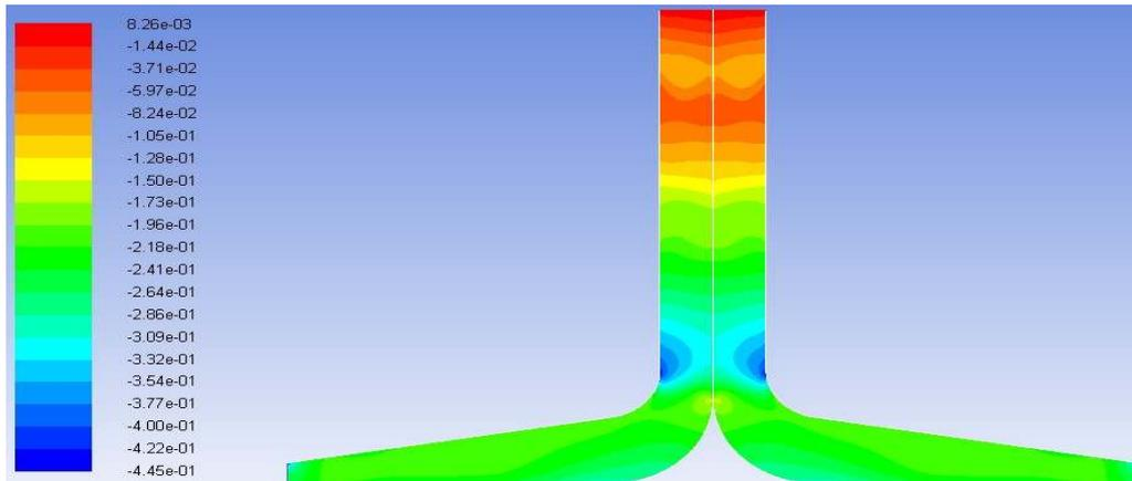
**Figure 5b.** Pressure contour maps of SUT plant at  $800 \text{ Wm}^{-2}$  at  $10^\circ$  canopy angle.
