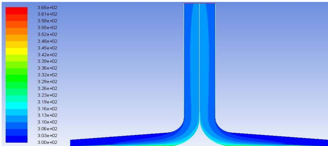
**Figure 3b.** Temperature contour maps of SUT plant at  $800 \text{ Wm}^{-2}$  at  $5^\circ$  canopy angle.
