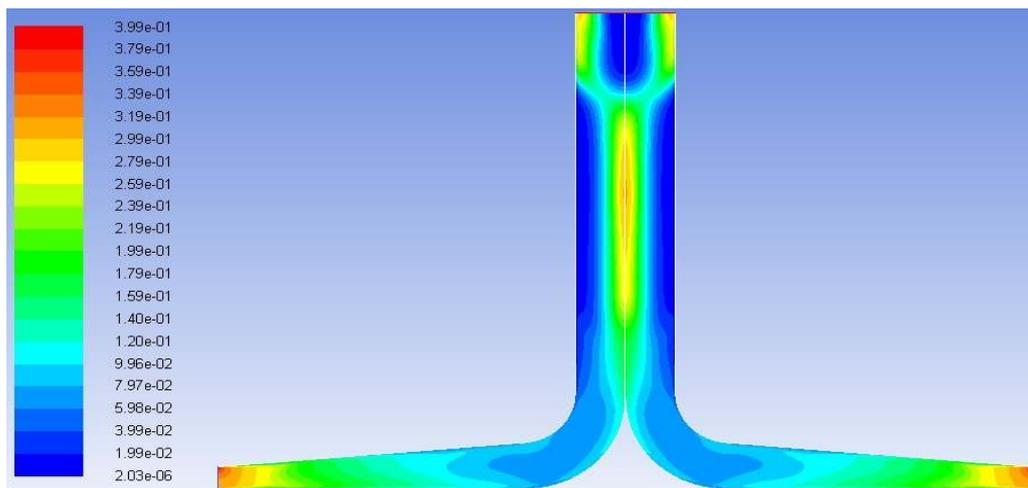
**Figure 2c.** Pressure contour maps of SUT plant at  $1000 \text{ Wm}^{-2}$  at  $5^\circ$  canopy value.
