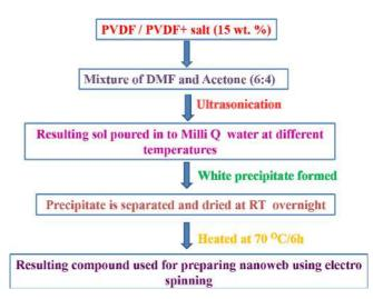
**Scheme 1.** Schematic procedure for the preparation of phase-separated PVDF.
