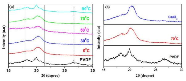
**Figure 3.** XRD analysis: Estimation of crystalline content in neat PVDF under varying phase-separation temperatures (a), and in 70 °C phase-separated PVDF-CaCl<sub>2</sub> (b).
