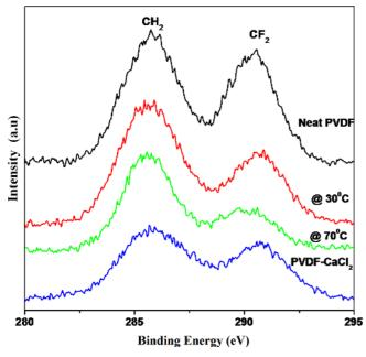
Figure 6. XPS of C1s core levels in neat PVDF, phase-separated PVDF (at 30 and 70  $^{\circ}$ C) and 70  $^{\circ}$ C phase-separated PVDF-CaCl<sub>2</sub>.
