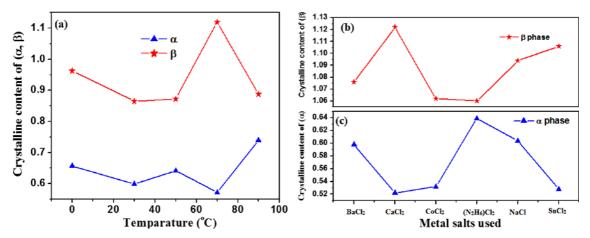
**Figure 2.** FTIR quantitative analysis: Estimation of crystalline content ( $\alpha$  and  $\beta$ ) in neat PVDF under varying phase-separation temperatures (a), and in 70 °C phase-separated PVDF containing different metal chloride salts (b), (c).
