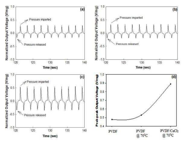
**Figure 8.** Normalized piezoelectric output voltage (V/mg) measured for electrospun samples: neat PVDF (a), 70 °C phase-separated PVDF (b), and 70 °C phase-separated PVDF-CaCl<sub>2</sub> (c). Peak-to-peak output voltage (V/mg) measured for the above samples (d).
