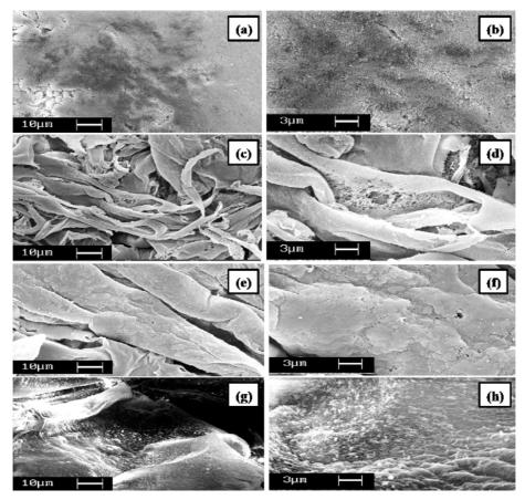
**Figure 4.** SEM images for neat PVDF (a), (b), 30 °C phase-separated PVDF (c), (d), 70 °C phase-separated PVDF (e), (f), and 70 °C phase-separated PVDF-CaCl<sub>2</sub> (g), (h) at two different magnifications, 500× and 1500×, respectively.
