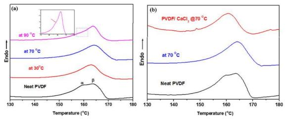
**Figure 5.** DSC curves of neat PVDF under varying phase-separation temperatures (inset showing a very small peak at 160.2 °C attributed to  $\alpha$ -crystalline phase) (a), and of 70 °C phase-separated PVDF-CaCl<sub>2</sub> (b).
