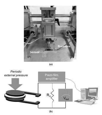
**Figure 7.** Setup for measuring dynamic pressure (a) and equivalent circuit diagram for measuring piezoelectric signal (b).
