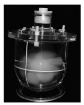
Fig. 5. Phantom used to verify a stereotactically guided conformal treatment plan. The phantom consists of an inner glass bulb containing the Acrylamide gel, which is surrounded by water in a Perspex container.)
