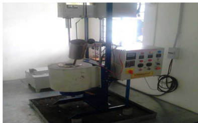
Fig 1 Stir casting setup used in experiment
