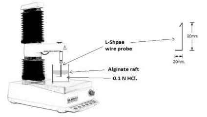
Fig. 1: Texture analyser: raft strength measurement. (TA. XT Plus, texture technologies, scarsdale, NY)
