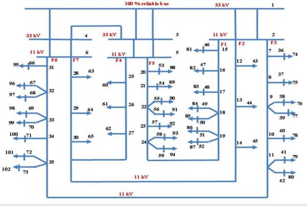
FIG. 3. Single line diagram for the RBTS Bus 4 distribution network.
