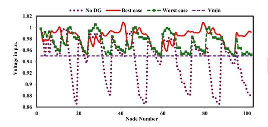
FIG. 13. Voltage profile plot for peak load condition.
