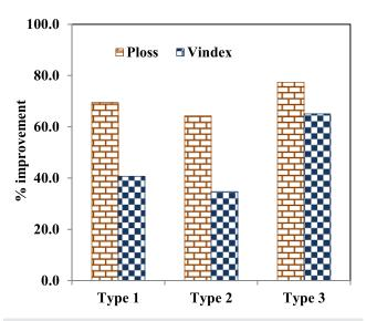
FIG. 11. Percentage improvement in real power loss and voltage deviation for commercial load.
