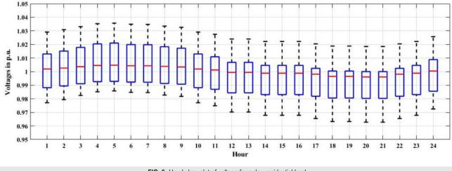
FIG. 6. Hourly box plot of voltage for a day-residential load.
