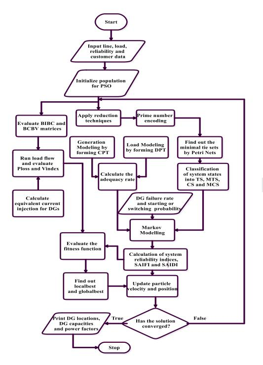
FIG. 2. Flow chart for the optimization algorithm.
