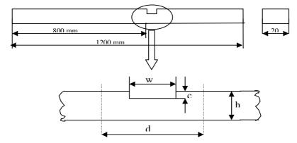
Figure 1. Beam model and Damage geometry
