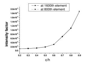
Figure. 5 Damage quantification using Intensity factor for different damage cases (c/h=0.2 to 0.9)
