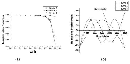
Figure 2. (a) normalized natural frequencies different damage cases for first three modes shapes (b) First three mode shapes
