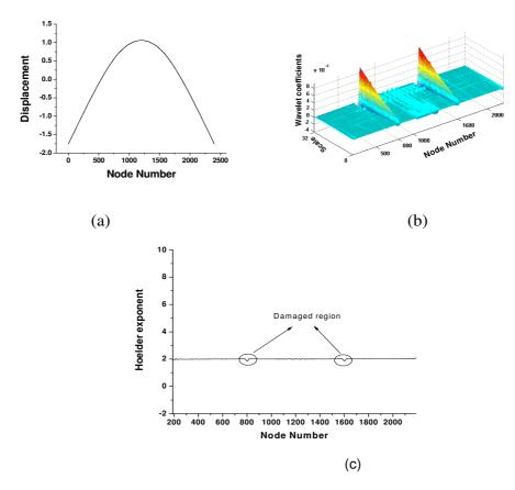
**Figure 4.** (a) Fundamental mode shape for damage case c/h=0.5 (b) 3-D Wavelet plot in Scale-translation plane (c) Hoelder exponent along the length
