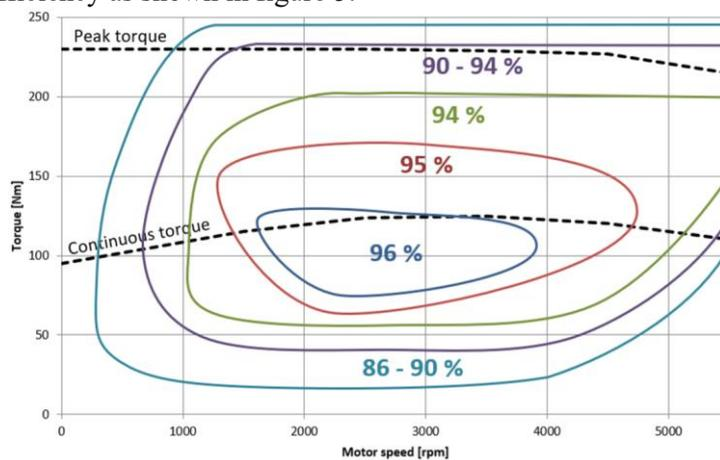
**Figure 4.** Efficiency map of Emrax 228 motor.
