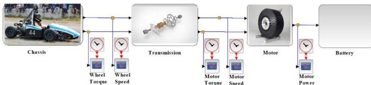
**Figure 1.** Scilab Model of formula student electric vehicle.
