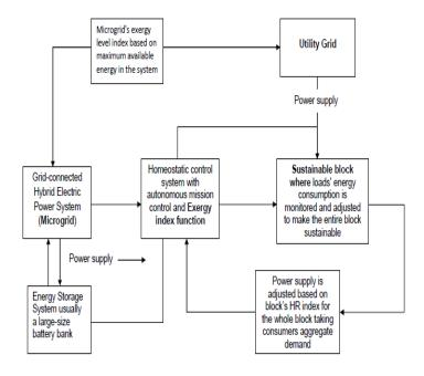
**Fig.1**. A particular example of the homeostatic control (HC) model for SHES. Here both energy and exergy management are built in the SHES to enable resilience and sustainability [10,18,19,21,22]. Source: owned elaboration
