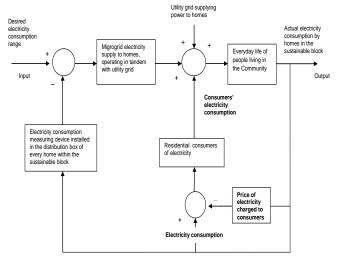
**Fig.3**. Flow diagram depicting the drivers of homeostatic control strategies to ensure efficient electricity supply and demand equilibrium based on energy and power consumption ranges per home consumers [10]. Source: owned elaboration.
