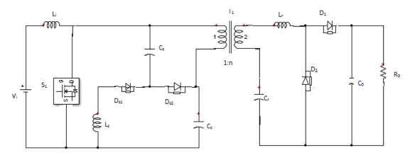
Figure 1. Proposed ZCS-ZVS Converter
