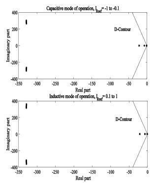
Fig. 7: Locus of eigenvalues of STATCOM with optimal controller parameters.
