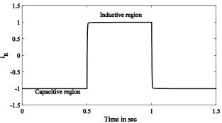
Fig.8: Step response of STATCOM with optimal controller parameters.
