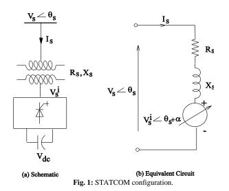
The converter of STATCOM is usually a multilevel or multi-pulse configuration. In a three-level converter with fundamental switching frequency, the magnitude of converter output voltage can be controlled by modulating the dead angle  $\beta$  [20], [21]. Also, the three-level configuration of converter minimizes the harmonic distortion on the ac side [2], [19], [21] and [22].
