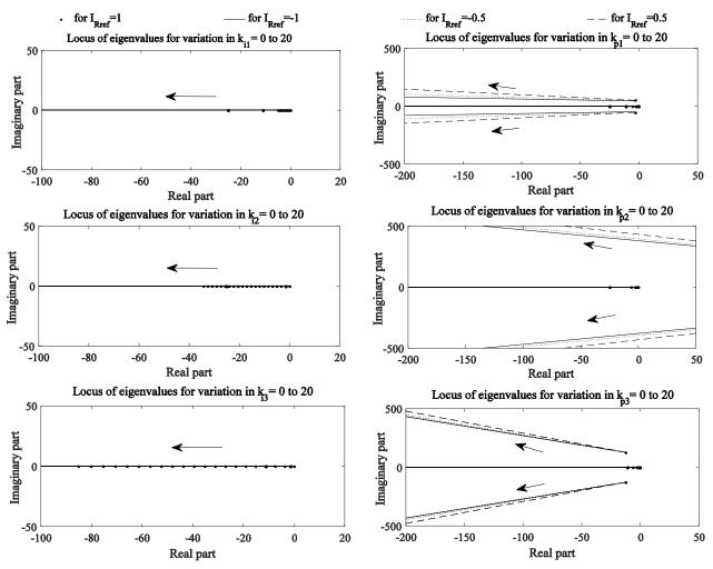
Fig. 3: Locus of the eigenvalues with the variation in control parameters for capacitive and inductive modes of STATCOM.
