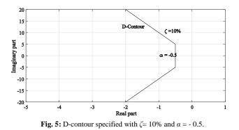
When the location of all the eigenvalues are in the left side of the contour shown in Fig.5, the conditions on  $\zeta$  and  $\alpha$  are met and also guarantees a well damped response for small disturbance. The contour which is shown in Fig.5 is referred as the D-contour [2], [25].
