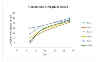
Figure 3. Compressive Strength with M Sand.
