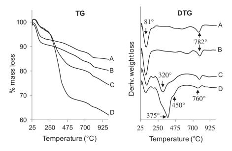
Fig. 6. Thermogravimetric and differential thermogravimetric patterns of (A) bentonite, (B) bentonite-oil, (C) bentonite-PK, and (D) bentonite-oil-PK.
