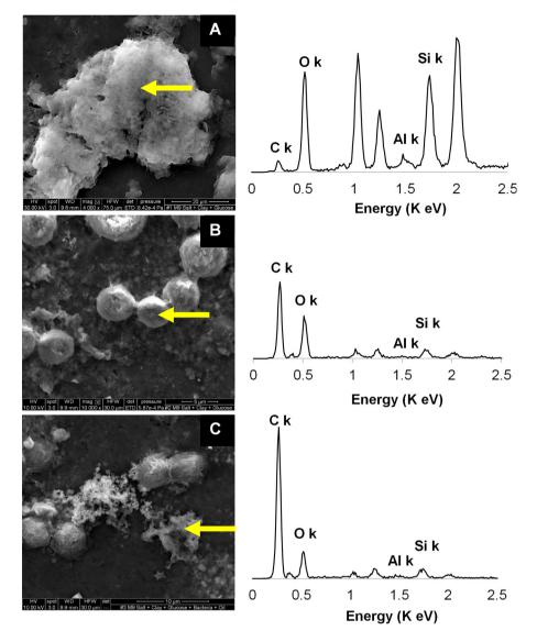
Fig. 2. SEM micrographs of clay-bacterial interactions and the corresponding EDX spectra from the arrow-indicated selected spots: (A) only bentonite, (B) bentonite-based PK agglomerates, (C) bentonite-oil-PK agglomerates and films.
