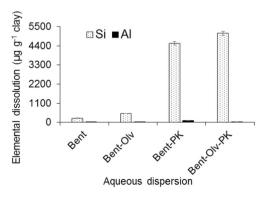
Fig. 3. Si and Al dissolution from bentonite into the culture media.
