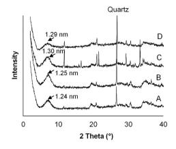
**Fig. 4.** XRD patterns of (A) bentonite, (B) bentonite-oil, (C) bentonite-PK, and (D) bentonite-oil-PK.
