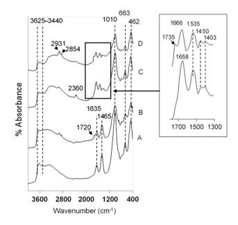
**Fig. 5.** FTIR spectra of (A) bentonite, (B) bentonite-oil, (C) bentonite-PK, and (D) bentonite-oil-PK.
