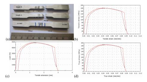
Fig.5.(a) As- tested Tensile Specimens (b) Tensile stress Vs Tensile strain (c) Load Vs Tensile extension (d) True stress Vs True Strain
