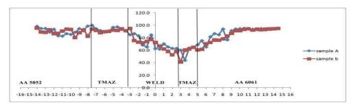
Fig.6. Hardness plot of Sample A and B
