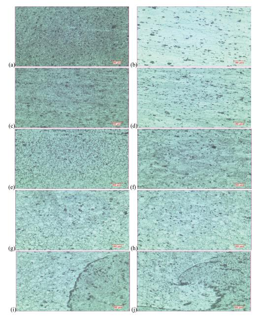
Fig. 4. Microstructures taken at the different zones of the welded Sample A and B (a)Base Metal of AA5052 (b)Base Metal of AA6061(c) HAZ of AA5052 (d)HAZ of AA6061(e)TMAZ of AA5052(f)TMAZ of AA6061(g)Weld region of Sample A (h) Weld region of Sample B(i)Interface in Sample A(j)Interface in Sample B.
