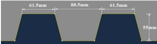
Figure 2. Dimensions of the profiled sheet
