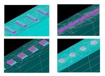
Figure 3. Meshed sheets clockwise from top left: with rectangular horizontal, rectangular vertical, circular and square embossments
