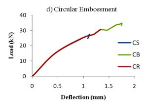
Figure 10. Comparison of load deflection curves for different sized embossments of circular shape
