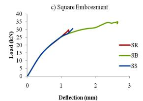
Figure 9. Comparison of load deflection curves for different sized embossments of square shape
