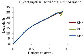
Figure 7. Comparison of load deflection curves for different sized embossments of rectangular shape horizontally aligned
