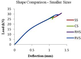
Figure 12. Comparison of load deflection curves for different shapes with smaller sizes
