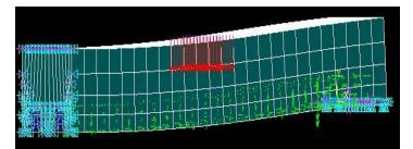
Figure 6. Deflected shape of composite slab after reaching ultimate load
