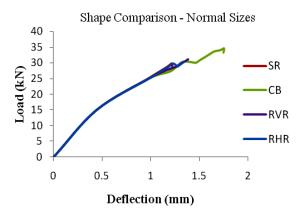
Figure 11. Comparison of load deflection curves for different shapes with normal sizes
