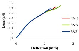
Figure 8. Comparison of load deflection curves for different sized embossments of rectangular shape vertically aligned
