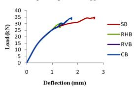
Figure 13. Comparison of load deflection curves for different shapes with bigger sizes
