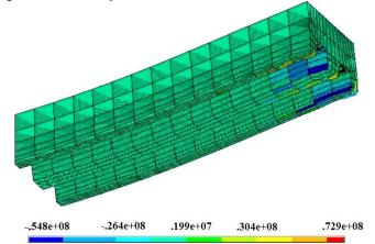
**Figure 14.** Longitudinal Shear Stress Plot for Slab with Square Bigger Type Embossment; values shown on scale in N/m<sup>2</sup>
