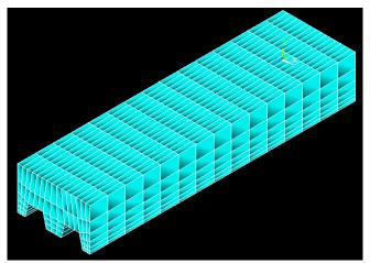
Figure 5. Elemental plot of the composite slab
