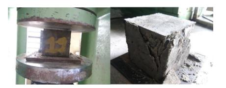
Figure 1. Testing and Failure Pattern of specimen
