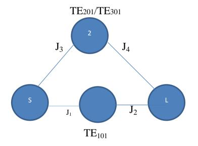
Figure 2. Circuitry representing the generated SIW cavity
