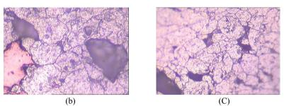
Figure 1: (a) 5% egg shell by wt; (b) 10% egg shell by wt;(C)15% egg shell by wt
