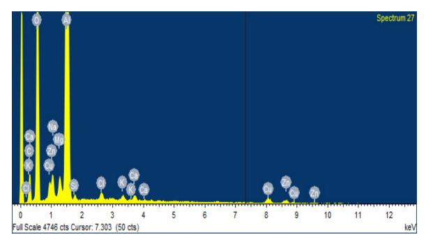
Figure 7: EDAX microstructures of Al6061 + 15% egg shell.
