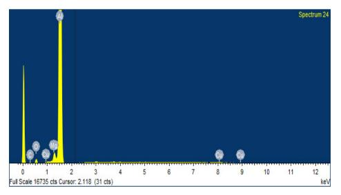
Figure 3: EDAX microstructure of Al6061 + 5% by wt egg shell
