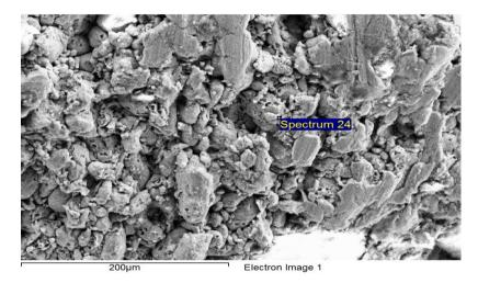
Figure 2: SEM image of Al6061 + 5% by wt egg shell
