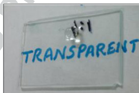
Figure 1. Photograph of water droplet on the transparent and superhydrophobic polyamide 12-SiO 2 (1:4) coating on glass slide.
