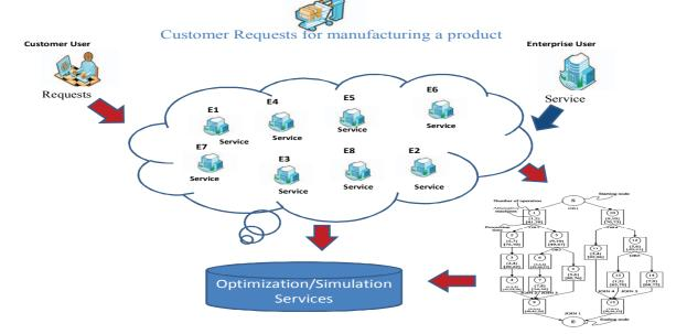
Figure 1 Networked manufacturing system architecture.
