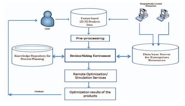
Figure 3 Web enabled system architecture.
