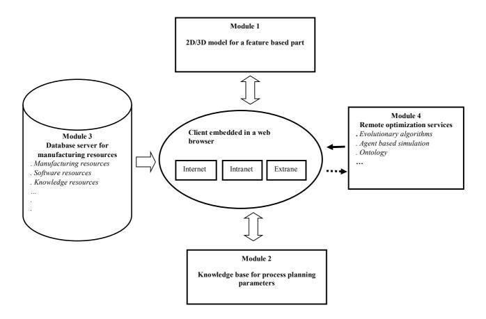
Figure 2. Modelling schema for the Functions of web-based system.
