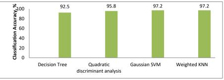
Figure 3. Comparative performance of the four best classifiers used for weld defect identification.
