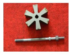
Fig. 12. Stator lamination and shaft with key.
