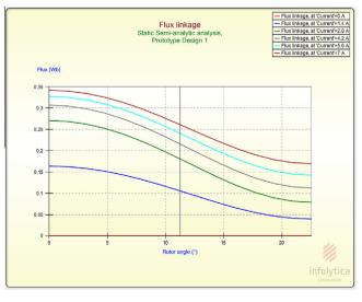
Fig. 5. Current - flux linkage characteristics.
